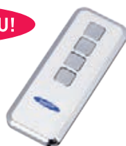
Handsender Mini-Novotron 524 Design 4-Kanal, 433 MHz, KeeLoq-Wechselcode
